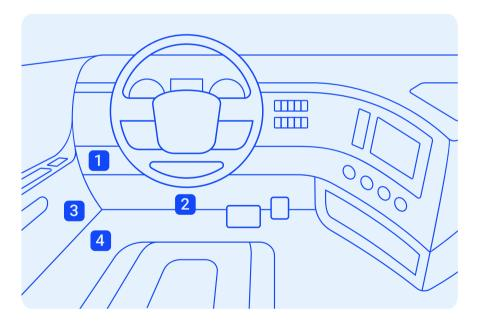
Attach the device to the diagnostic port of the vehicle.
